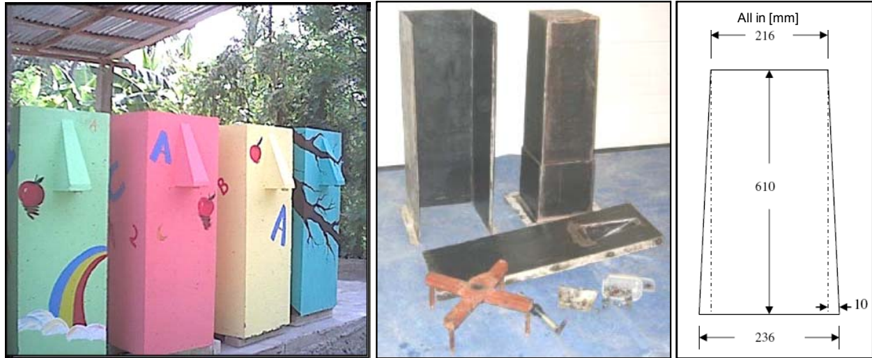
Figure 4-2 Concrete Rectangular BSF; Picture of Concrete BSFs in Haiti (left), Picture of Inner and Outer Mold (middle), Dimension of the Walls of the Inner Mold (right)
