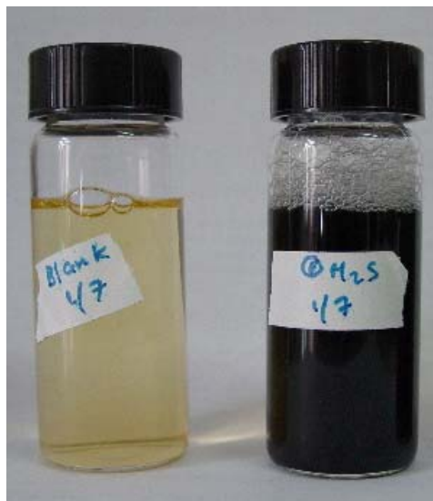
Figure 3-4 H 2 S Bacteria Presence/Absence Test
