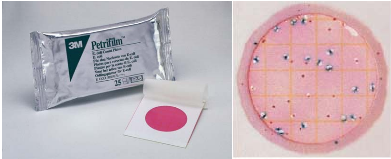
Figure 3-2 3M Petrifilms (left), Red and Blue Colonies with Bubbles (right) (Source: http://solutions.3m.com/wps/portal/3M/en_US/Food_Industry/Home/Prod_Info/Products/Microbiology/Petrifilm_Plates/ )
