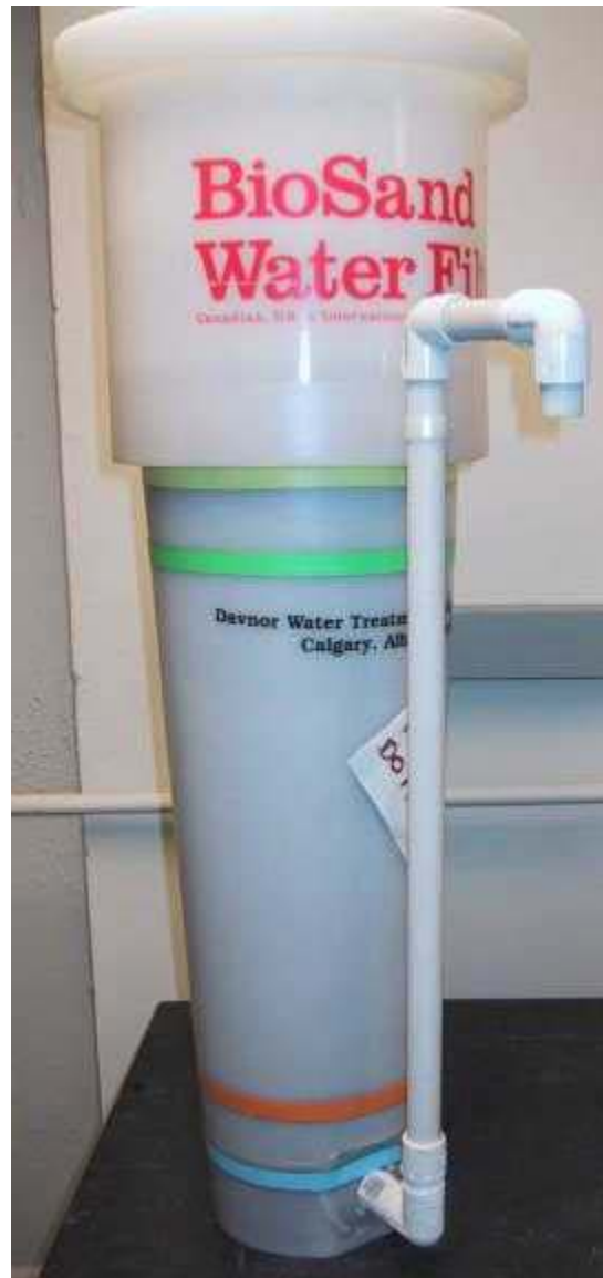
Figure 4-4 Picture of the Plastic Davnor BSF
